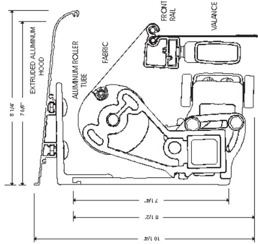
pitch to the desired position. Refer to the pitch chart on this page for minimum pitch recommendations. Adjust all arms until the front rail is level. **Securely** tighten the two nuts located on the side of the shoulder joint
